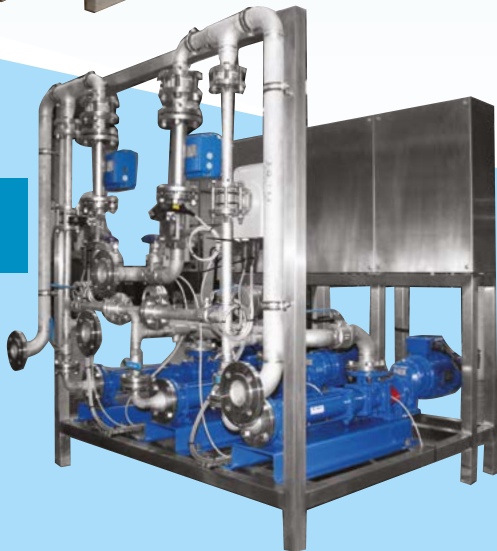
Bentonite make-up system
