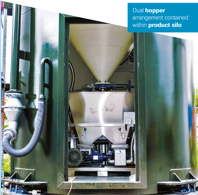
Bespoke dosing and pump skid units for Bentonite system
